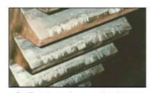
Scuffing is a damage related to a metal/metal contact during the meshing resulting in tearing of material. Scuffing occurs when the lubricating film breaks. They can be localized at a precise point, on the sliding zones only or finally on the whole surface.
